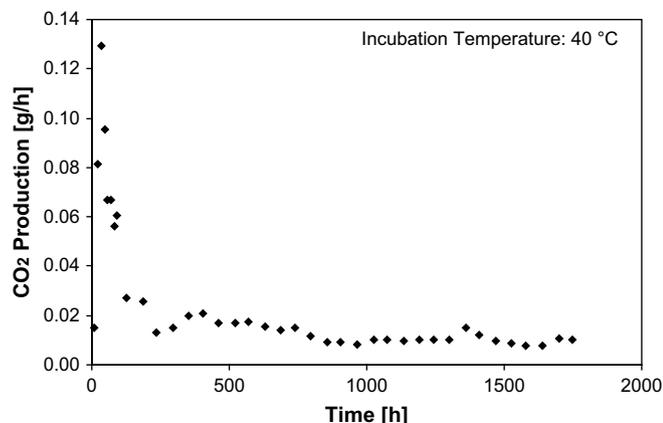
Fig. 8. Carbon dioxide production over time during the incubation of pine wood chips at a temperature of 40 °C.
