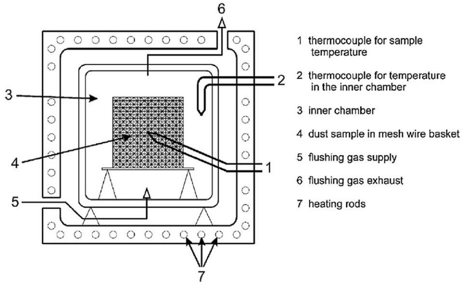
Fig. 1. Hot storage test set-up.
