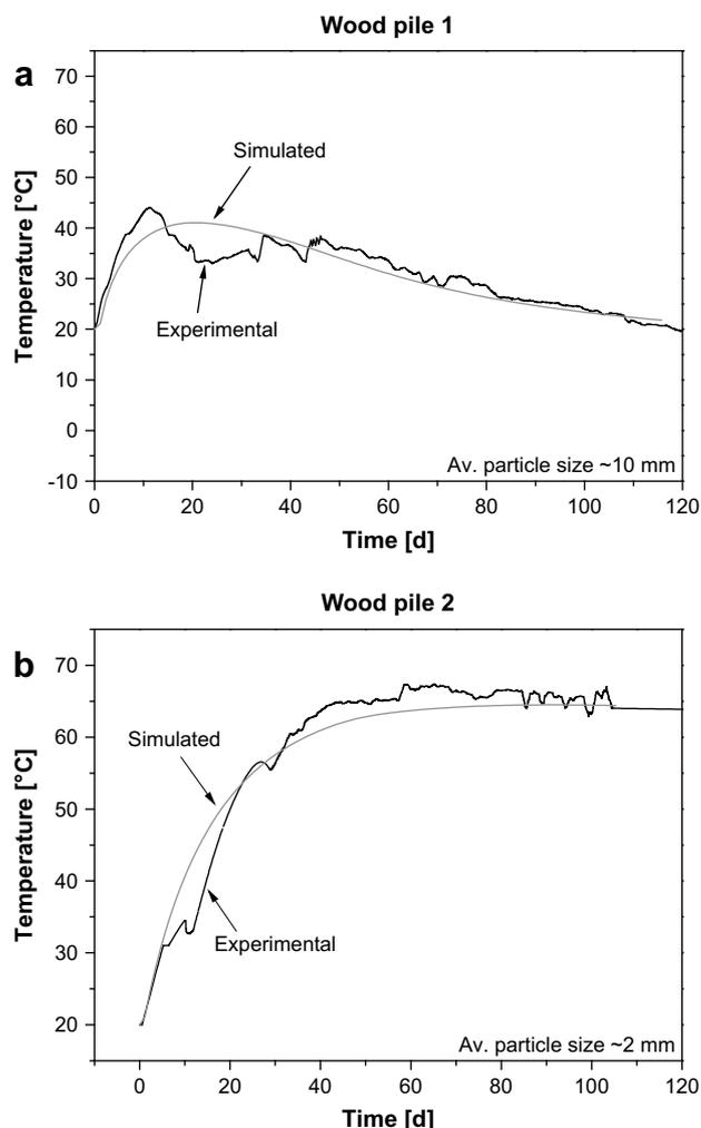
Fig. 9. Temperature evolution in the center of the Wood Piles 1 (a) and 2 (b): model predictions vs. experiments.
