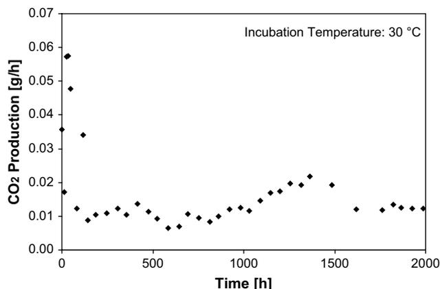
Fig. 7. Carbon dioxide production over time during the incubation of pine wood chips at a temperature of 30 °C.
