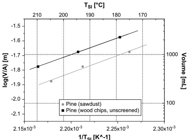
Fig. 2. V/A dependence of the self-ignition temperature for pine wood.
