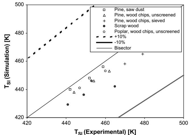
Fig. 6. Comparison of the numerically simulated and experimentally determined self-ignition temperatures for the investigated woods.
