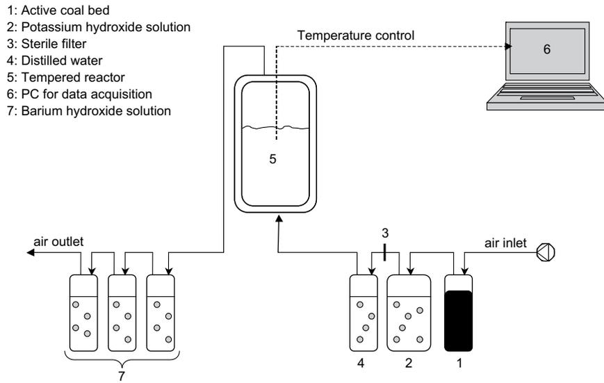
Fig. 4. Schematic drawing of the respiratory test.
