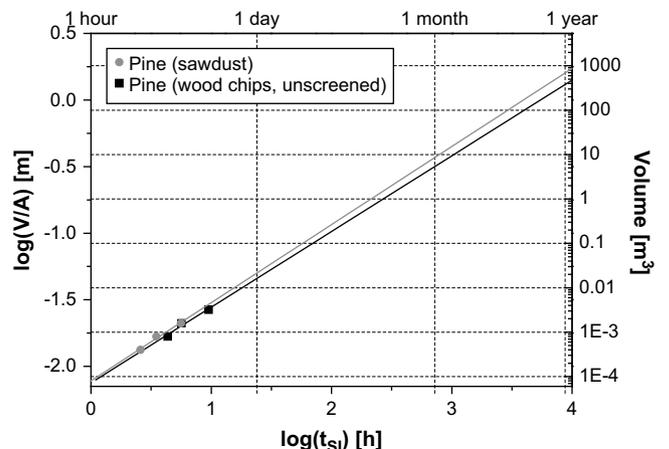
Fig. 3. Extrapolation of the induction time to self-ignition for pine wood.
