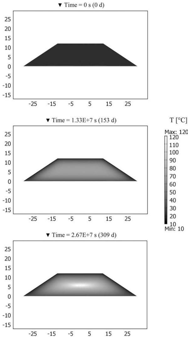
Fig. 10. Study of the self-ignition of a pine wood pile (height = 12 m, width = 60 m, material stored at an ambient temperature of 15 °C).
